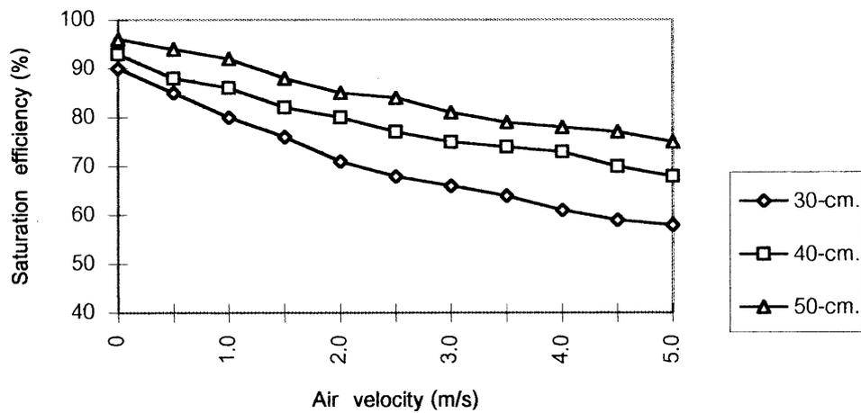
Fig. 7. Evaporative cooler effectiveness for various pad thickness and air flow.
