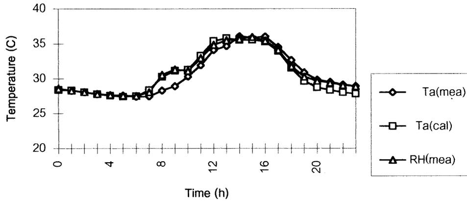
Fig. 5. Simulated and measured temperature of the mushroom house.
