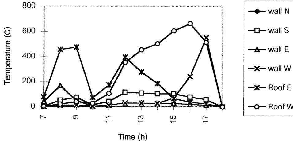
Fig. 3. Solar radiation on the walls and the roof. (Calculated from measurements on a horizontal plane; 25 March 1996.)
