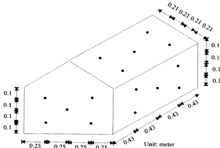
Fig. 2. Schematic representation of the experimental mushroom house without EC. (● Location of temperature measurement on roof and wall.)
